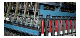
centred, spindles are correct centred (for longer lifetime and better yarn/hairiness). Use antiballoon to control yarn tension and decrease contact with separators;
