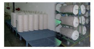
However, if the mills are using German technology which has the chute feed system, the handling of laps does not remain a problem. Chute feed is direct from the opening line, hence there is no lap waste (first meter), no problem of damage to the lap, no left over, and no labour involved. It is a relatively easy machine giving high production. This is also essential if the mill uses high production cards.
