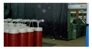
In the carding section, if the sliver breaks for some reason, the whole can should be changed or else the manual handling of the sliver will affect layers of the sliver in the drum and hence the quality of yarn produced.
