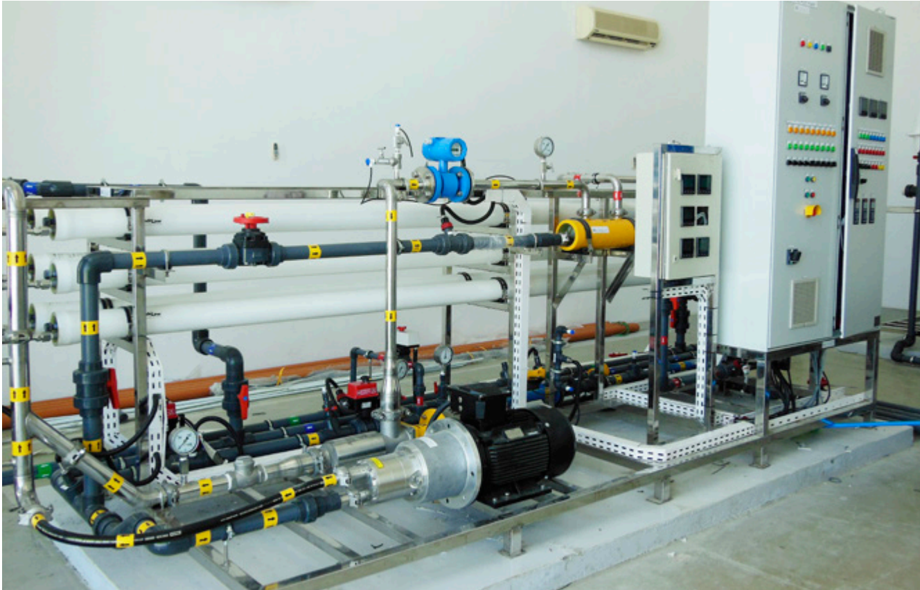
Reverse osmosis pilot plant at MEDRC facilities, North Al-Hail, Oman
