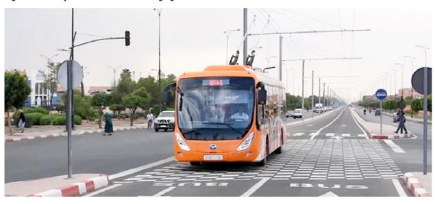
Figure 17: Trolley bus with in-motion charging in Marrakech
