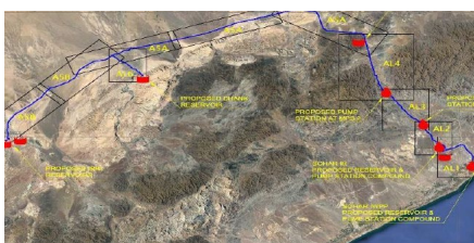
Project Master map (pipeline route from Sohar desalination plant on the Oman Sea to Ibri City)
